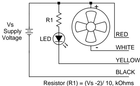
Figure 1. Connection diagram for LED alarm indication.
