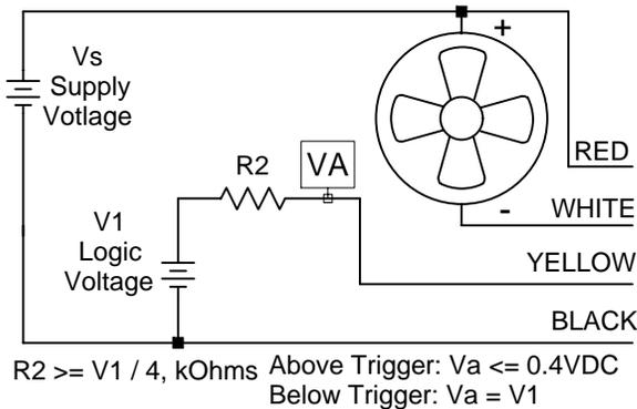
Figure 2. Connection diagram for logic circuit alarm indication.
