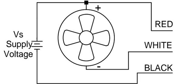
Figure 3. Connection diagram when the temperature alarm output is not used.
