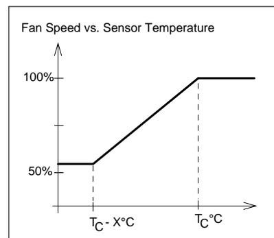
Figure 4. Fan speed vs. sensor temperature
